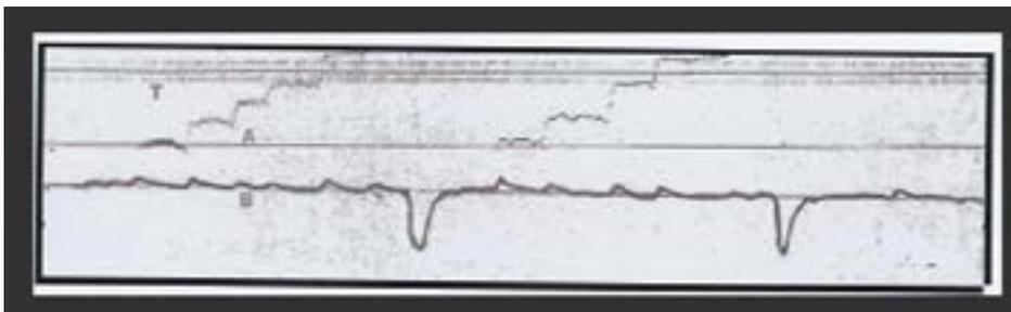
Fig 4. Signal amplitudes shown over time for a subject reading two lines of text. Eye position (A) shows upward, stair-step signature as eyes move from word to word; downward return-sweeps move eyes to next text line. Polarity of differentiated position signal (B) was reversed in keeping with actual direction of EMs. Timing signal (T) marks one-second intervals.<sup>19</sup>
