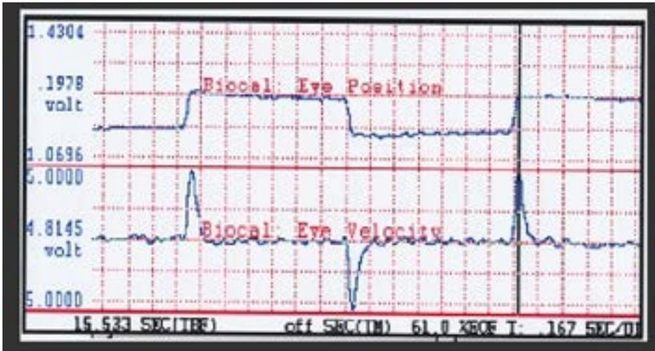
Fig 2. Signal voltages over time (in sec) for eye position using DC amplifier and saccadic velocity using AC amplifier; subject fixated on two letters in succession appearing at left and right margins of text screen. Fixation time is the inter-saccadic interval on velocity channel. Data set is from a Beckman recorder with signals ported to a Dataq digitizer with Windaq viewer.<sup>17</sup>
