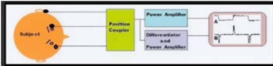
Fig 3. Schematic diagram of biocal signals from electrode placements, to position coupler, to amplifiers, and finally to a dual-channel, monitor, which displays eye position (A) and saccadic velocity (B).<sup>20</sup>
