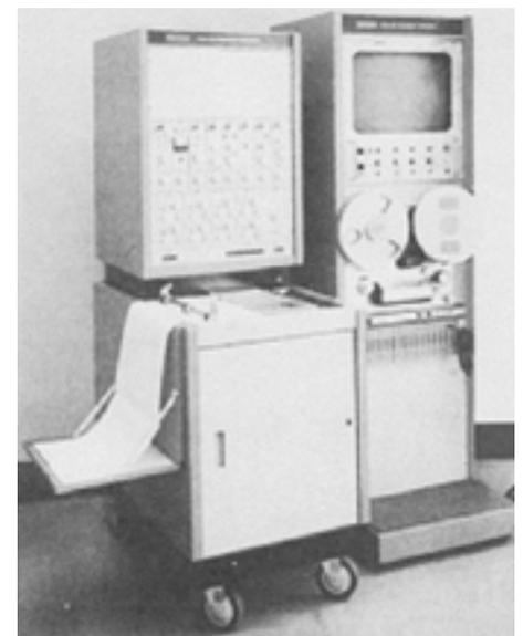
Fig 1. A paper recording, monitoring and storage system for biomedical data consisting of an ink-writing polygraph (left), monochrome monitor (top right) with a multitrack, magnetic tape recorder bottom right; adapted from the Beckman Historical Collection.<sup>13</sup>
