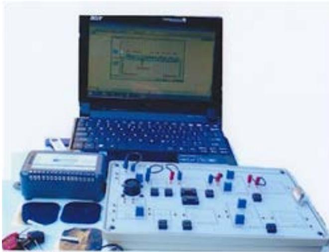
**Fig 5. A sub-notebook PC from Acer (left); Dataq's dual-channel, data-logger (center); Heathkit's dual-channel, EOG unit (right) with electrode patches and cables (foreground) comprise a compact, student-friendly, system for empirical studies of reading behavior.<sup>35</sup>**
